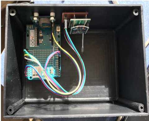
Figure 30. Circuit box coordinator meteorological station and receiver Xbee.
