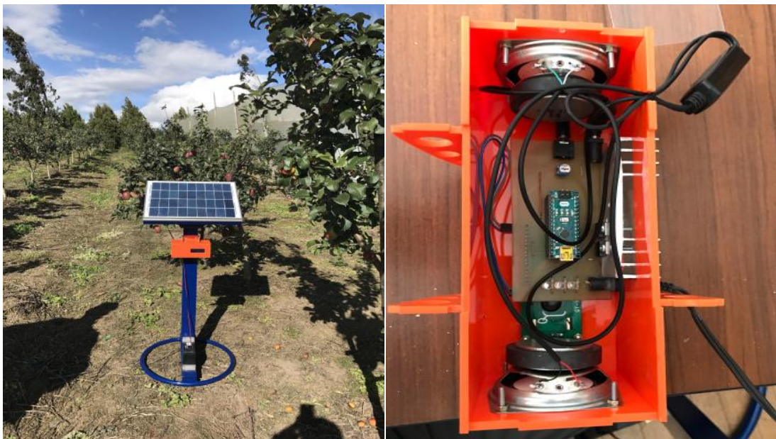
Figure 41. Pest management device showing the circuit and its internal and external components in an apple crop of the Juan de Castellanos University Foundation in Soraca Boyacà Colombia.
