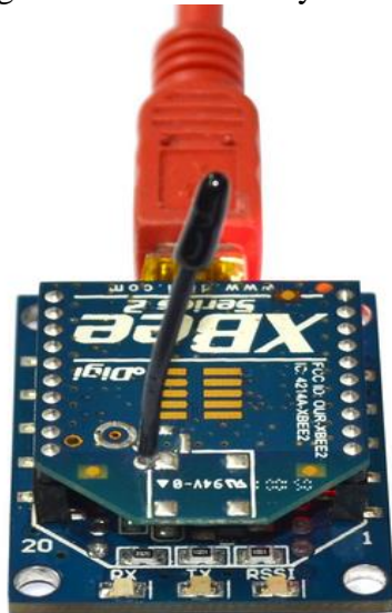
Figure 20. Xbee programmer to assign router and coordinator in XCTU software
