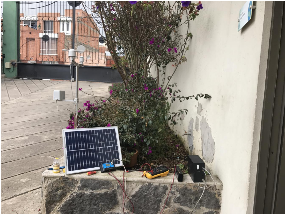
Figure 27. Tests meteorological station at the Juan de Castellanos University Foundation Headquarters with the router circuit and coordinating circuit with data transmission.
