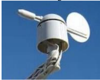
Figure 10. Vane of variable resistance
