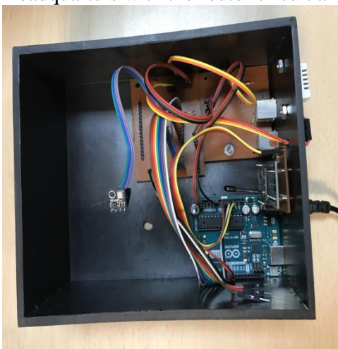
Figure 27. Tests meteorological station at the Juan de Castellanos University Foundation Headquarters with the router circuit and coordinating circuit with data transmission.
