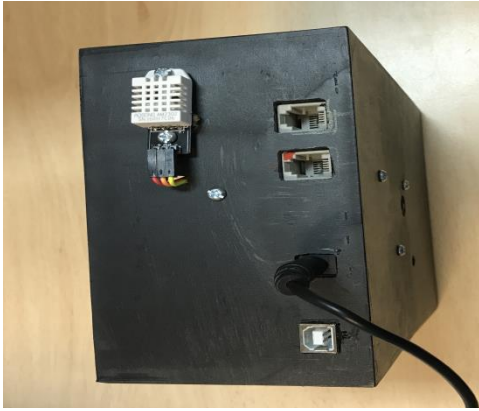
Figure 29 Box router circuit with sensor of Temperature, Humidity and Inputs sensor of publiccity, speed of wind and direction of wind.
